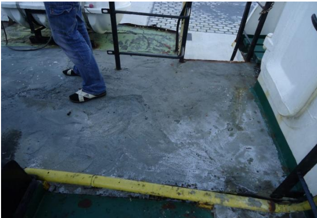
Deck plating of the bridge deck (around the funnel) was covered by cement.
