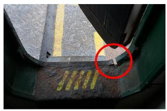
Improvised electrical cables crossing emergency generator room weathertight door.
