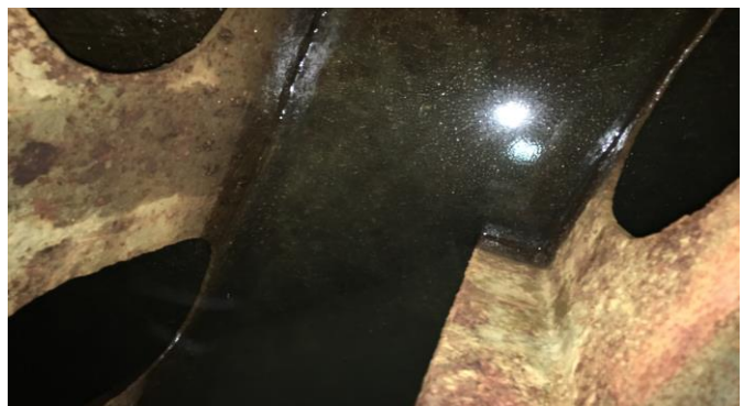
Picture n. 6: Oil in WBT (Aft Peak Tank)
