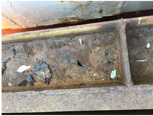
Picture n. 4: Hatch cover edge holed by severe corrosion.
