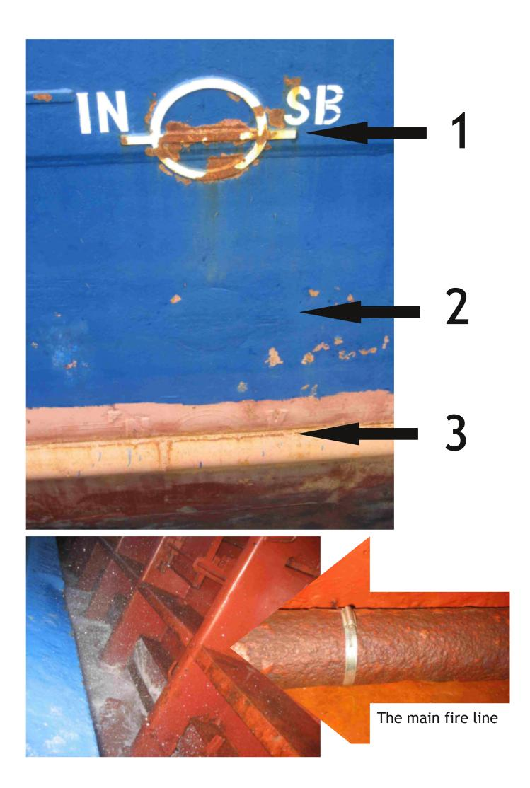
• main fire line is holed in main deck and heavy leaking (temporary repairs by clamps are noted);
