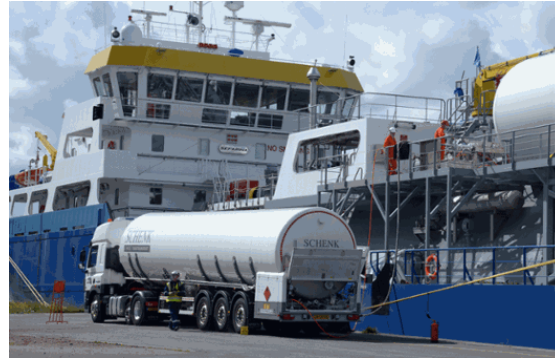
Fig.2.6 – Truck-to-Ship LNG bunkering.
