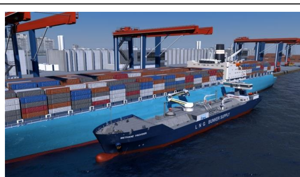
Figure 12.12 – Ship-to-Ship (PTS) Bunkering.
