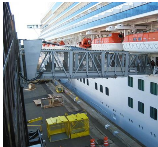
Figure 11.4 – Enclosed Gangway to access a passenger ship at main deck level – enclosed gangways have the potential to protect passengers in the event of an accidental LNG release.
