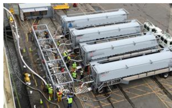
Figure 3.5 – LNG Bunkering interface – manifold connection
