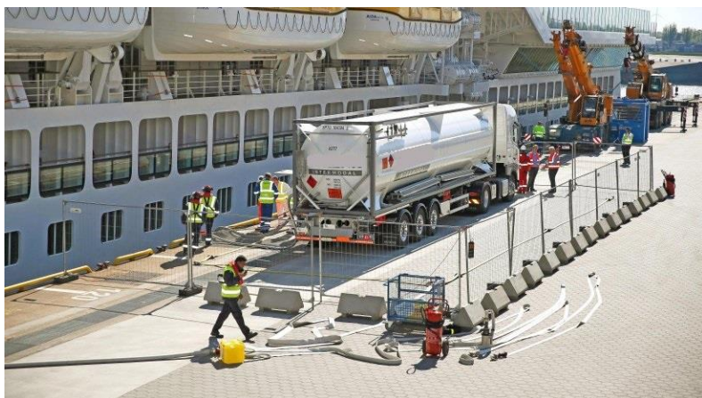
Figure 3.12 – LNG feeding operation directly into LNG dual fuel engine inside the ship
