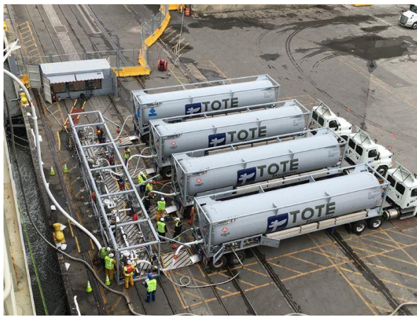
Figure 12.5 and 12.6 – TTS Bunkering by multiple trucks, via common manifold. It can be seen how the complexity of the operation is increased, not only with significant number of connection to common manifold but also with a significant number of personnel. To the technical challenge there is also an organizational one.
