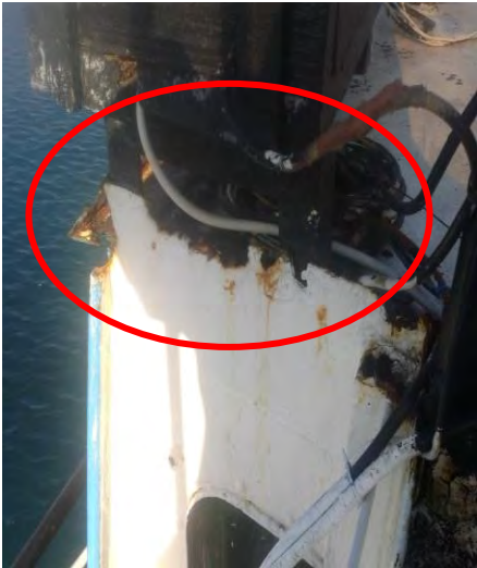
Various cracks / bends and holes, on the metal plate all around the monkey deck
