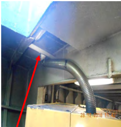
Alterations of the deck plate, in order to create access for the above pipes lines to the upper deck
