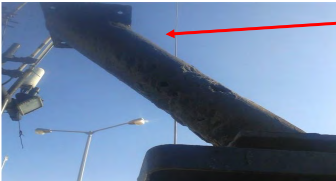
Various cracks / bends and holes, on the metal plate all around the monkey deck
