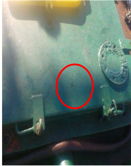
Holes on the cargo hold hatch (which was converted as cargo tank)
