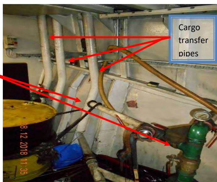
Ballast pump, connected with the cargo transfer piping system, modified as such to be able to transfer oil from the cargo tanks to the main deck and also overboard.
