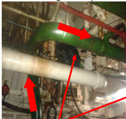
The piping from the suction pump (bilge) leading to the upper deck (overboard)
