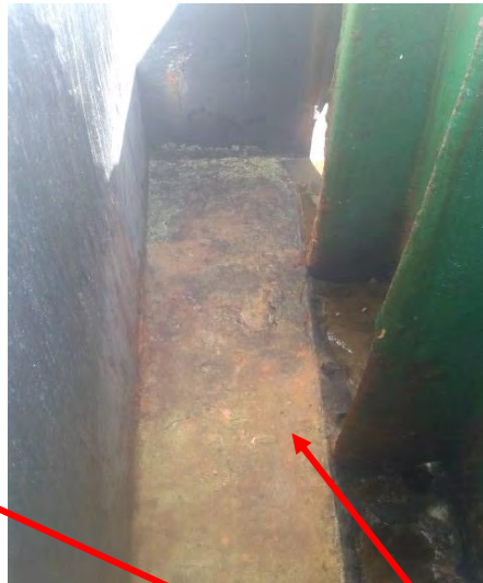
Holes on the cargo hold hatch (which was converted as cargo tank)
