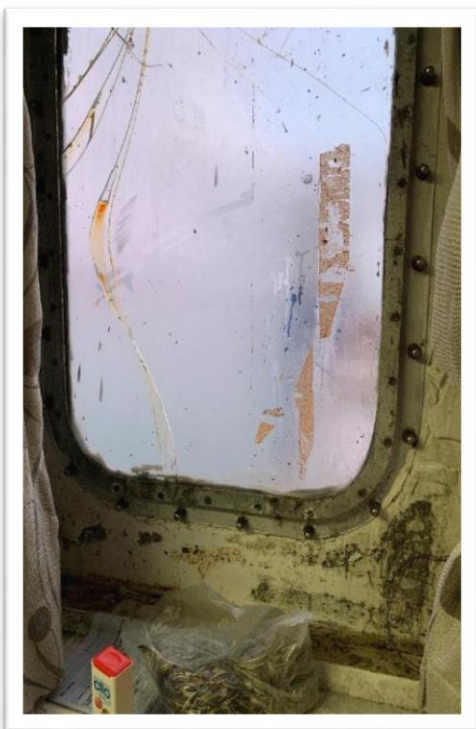
Picture 2: Cracked window inside 3rd Off. cabin
