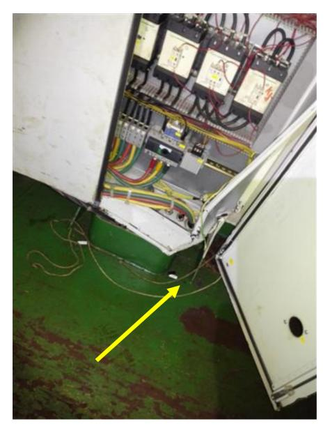
Because of the many unlashed drums, both mooring winch control cabinets were heavily damaged. The cabinets were impossible to be closed at all. Crew stated during interview that this had been known for a long time but no spare part orders were forwarded to the company at all. Due to these facts. all deficiency was recorded with ground for detention.
