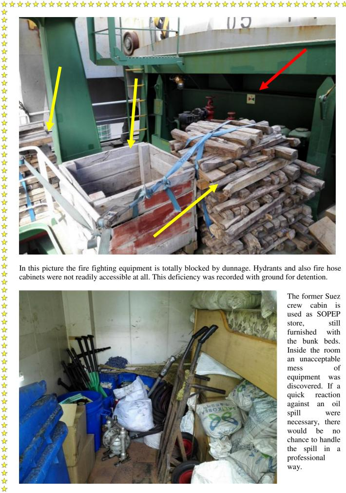
In this picture the fire fighting equipment is totally blocked by dunnage. Hydrants and also fire hose cabinets were not readily accessible at all. This deficiency was recorded with ground for detention.
